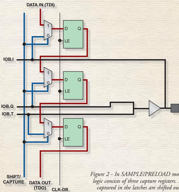
Figure 2 - In SAMPLE/PRELOAD mode, the scan logic consists of three capture registers. I/O signals captured in the latches are shifted out serially.
