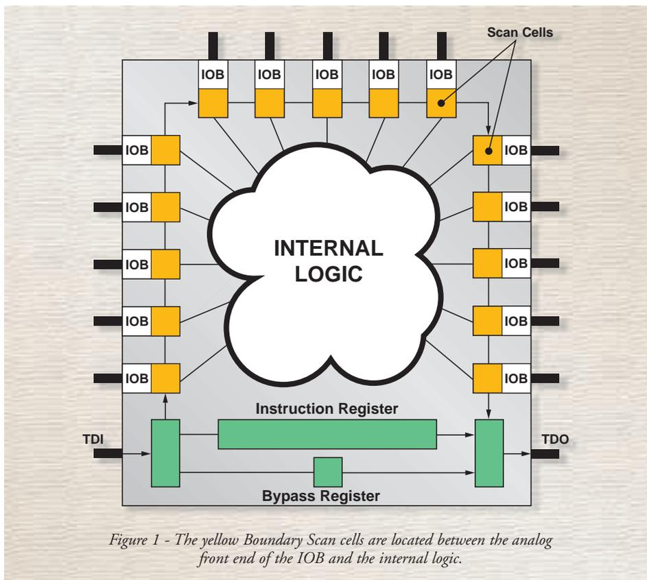
Figure 1 - The yellow Boundary Scan cells are located between the analog front end of the IOB and the internal logic.
